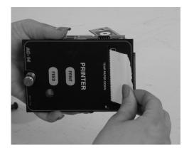
**2.** Pull paper out from front. Pulling paper from the back could tear paper and leave jammed section inside. Reload paper.
