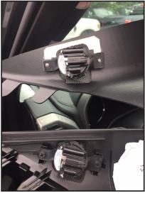
Insert screw into pillar, slide spacer over screw, align screw with snap nut and attach
