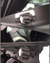
Insert screw into pillar, slide spacer over screw, align screw with snap nut and attach
