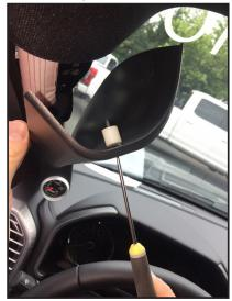
6) Connect speaker wire, insert bottom of pillar into dash area first.
