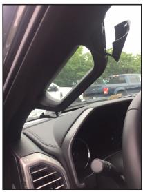
Install supplied snap nut into lower portion of slot
