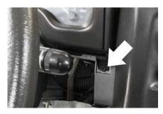
4) Remove the remaining two screws from the bottom of the factory bezel. They are located on the bottom left and bottom right of the factory bezel. Retain the screws, they will be reused in the installation of your new panel.
