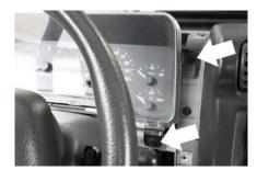
5) Remove the 4 screws securing the factory instrument cluster. These screws will not be reused.
