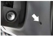
3) Remove the two screws that hold the dash panel below the steering column. There is one screw on each side; one near the headlight switch and one near the ignition switch. Retain the screws, they will be reused during installation.
