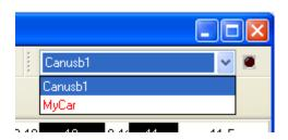
On legacy systems, when the CAN USB adapter is plugged into the PC, the active connection should show **Canusb1**.
