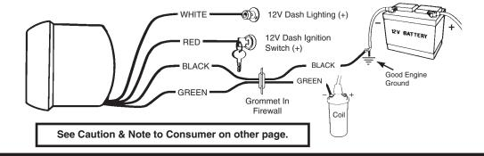
Figure B is for ignitions that provide a tach terminal, including **GM HEI**, and **MSD** (except **MSD-5**)
