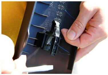
5. The safety strap is then removed from the factory pillar. The tab on the back is depressed and it slides right out.
