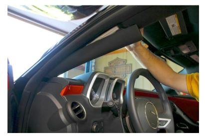
To start, pull the factory A pillar down. It pops out, but don't try to pull it all the way down.
