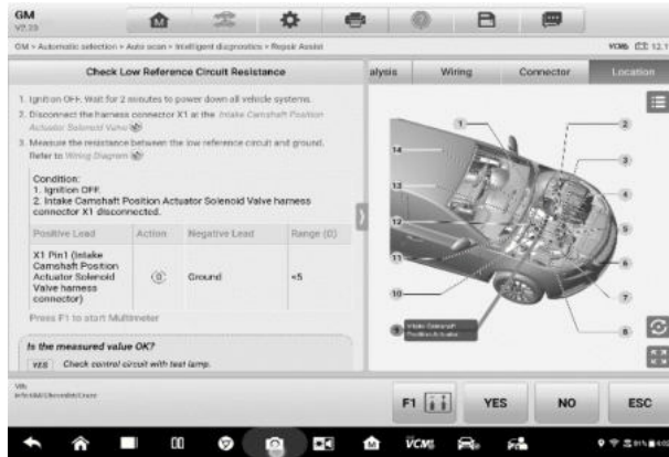
Figure 5-24 Sample Repair Assist Screen 5
