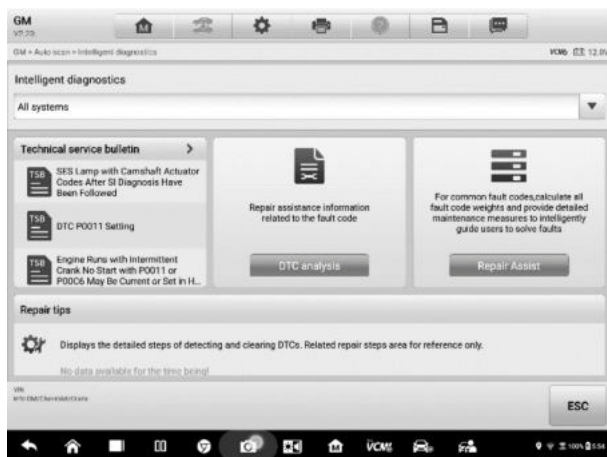
Figure 5-20 Sample Repair Assist Screen 1
