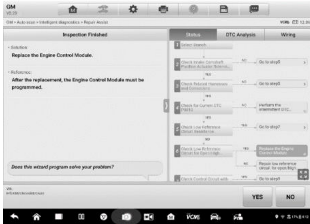
Figure 5-28 Sample Repair Assist Screen 9
