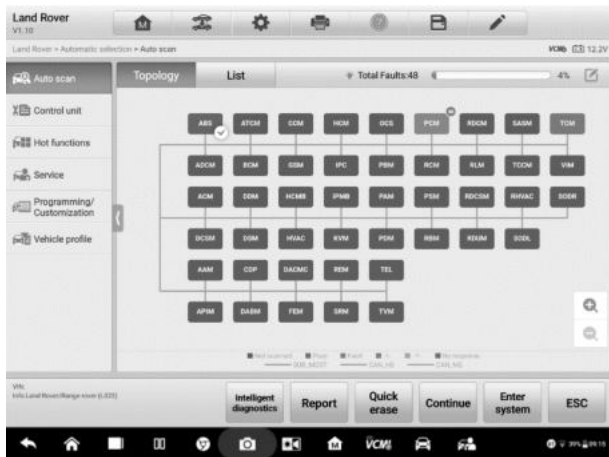
Figure 5-6 Sample Fault Scan on Topology Screen
