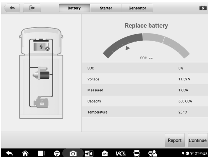
Figure 7-5 Sample Battery Test Results Screen
