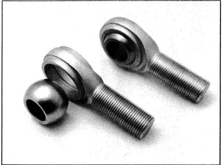
Finished ball with finished body of two piece full-swage rod end prior to assembly and finished unit.
