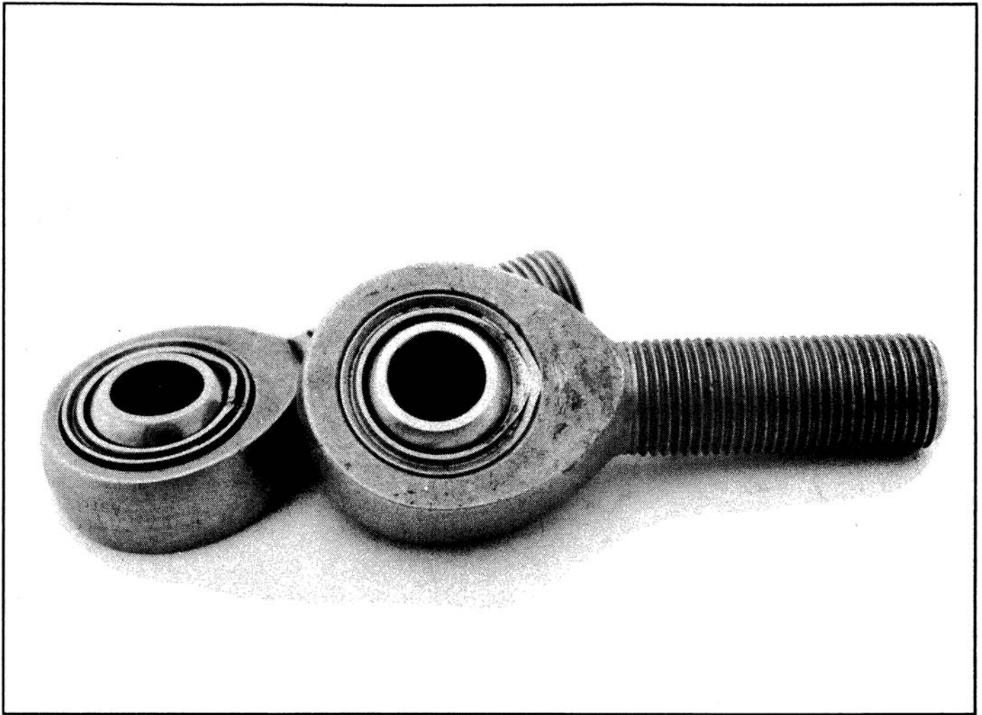
More damaged rod ends.
