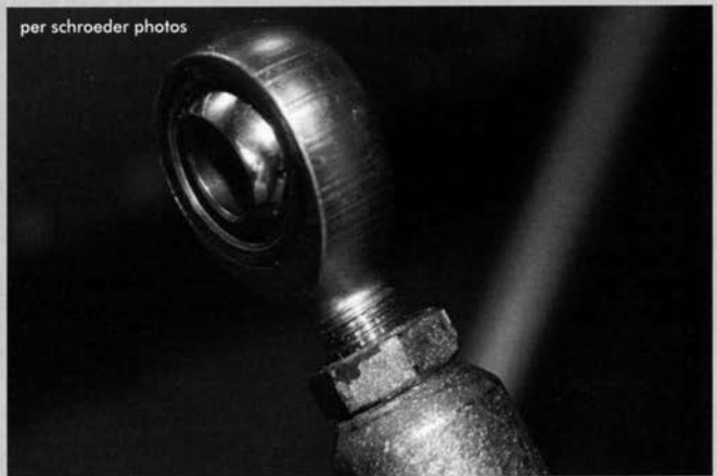
ABOVE: We replaced our old rod ends with brand-new hardware sourced from Aurora. BELOW: The LeGrand also uses a pair of rod ends to support the steering rack. In this case, we used lightweight aluminum pieces from Aurora. We also took a look at our gauges—or, rather, we tried to take a look at them, but they were too hard to read. A new Stack ST 1800 display unit was the solution. It's a customizable setup, and we specced our tachometer with a 15,000 rpm rev range. Our old muffler was too loud, so we swapped it with a new two-stage unit from Burns. This should keep us from raising the ire of the sound police.
