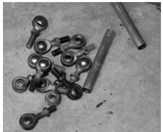
The old rod ends were worn, and we could feel that several had some play in them. Not good for a suspension!
