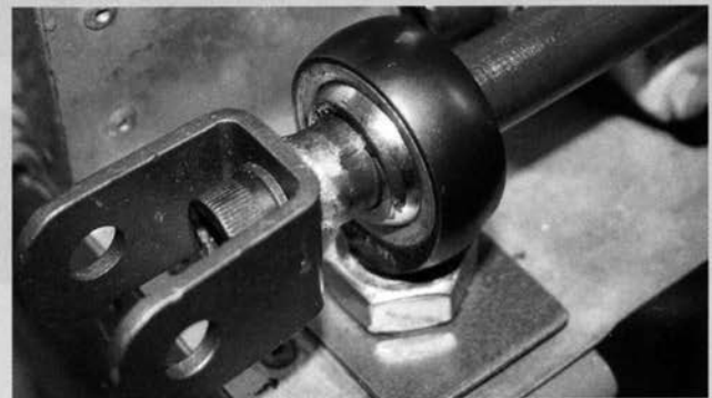
ABOVE: We replaced our old rod ends with brand-new hardware sourced from Aurora. BELOW: The LeGrand also uses a pair of rod ends to support the steering rack. In this case, we used lightweight aluminum pieces from Aurora. We also took a look at our gauges—or, rather, we tried to take a look at them, but they were too hard to read. A new Stack ST 1800 display unit was the solution. It's a customizable setup, and we specced our tachometer with a 15,000 rpm rev range. Our old muffler was too loud, so we swapped it with a new two-stage unit from Burns. This should keep us from raising the ire of the sound police.
