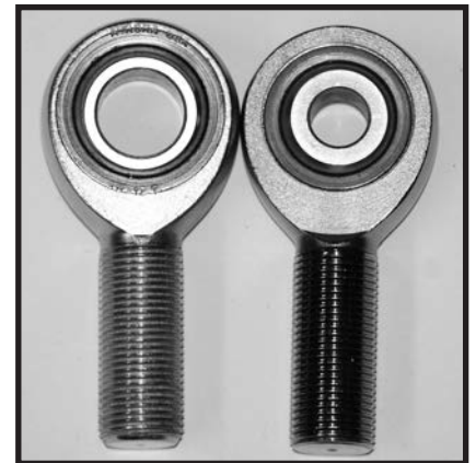
The rod end on the left is a standard configuration model, while the rod end on the right is a heavy duty model. The special HD model has a 1/2 inch bore while the standard version has a 3/4 inch bore. More in the text.
