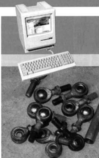
LEFT: During a wintertime work session, we found that most of our car's suspension joints were rod ends of various ages and conditions. We junked them all and ordered replacements. RIGHT: While our suspension was disassembled, we repainted the trailing links and control arms.
