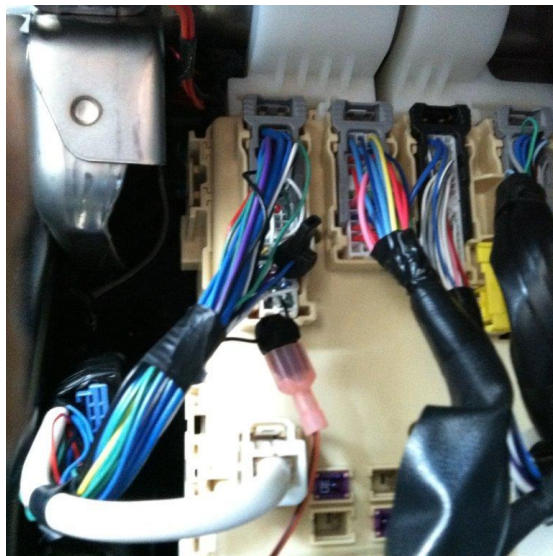
Picture 13A Connector 3A, pin 34 Orange-Black to Pin 34, Black wire
