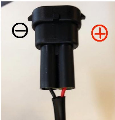
Picture 5 LED Fog lamp connector
