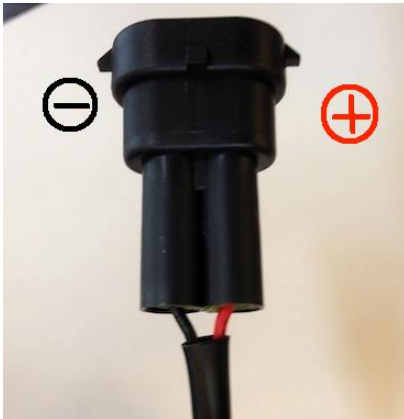
Picture 5 LED Fog lamp connector
