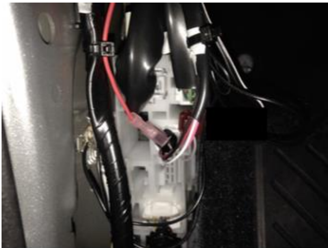
Picture 8: DRL red wire to connector (IC3, pin8)
