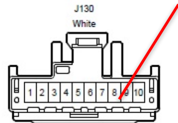
Picture 9: DRL red wire to connector J130 (light green wire)
