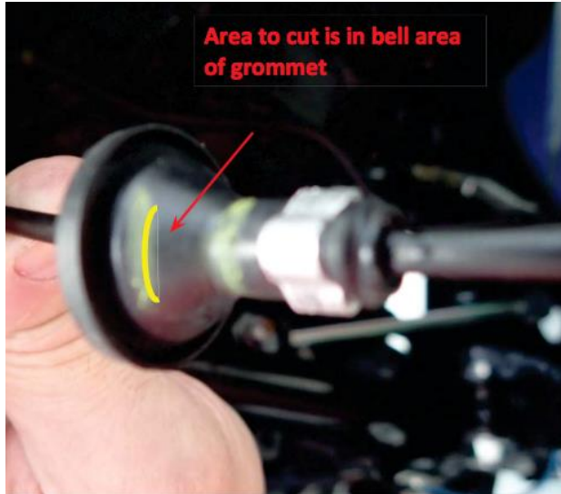
Picture 15C: Showing where to cut the grommet
