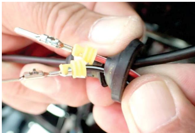
Picture 15E: Running the wires through the grommet
