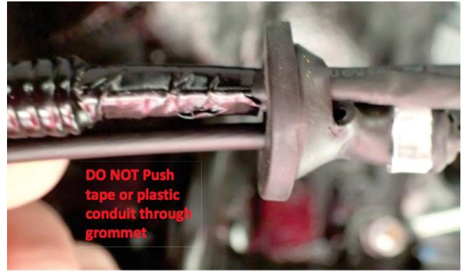
Picture 15F: do not push tape or plastic through grommet.
