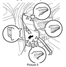
Remove left side switch panel: Remove switch knockout, then remove screw and claws securing panel (pictures 6 and 6A)
