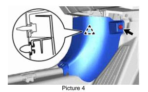
5. Remove side instrument panel. Using a pry tool, disengage the clips (picture 5)
