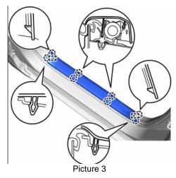
Remove the side kick panel by removing the clip (picture 4)
