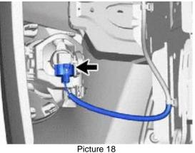
20. Remove the factory fog lamps, by removing the factory screw (s). Note: Factory screws will be used on installation. Do not discard them (picture 19).
