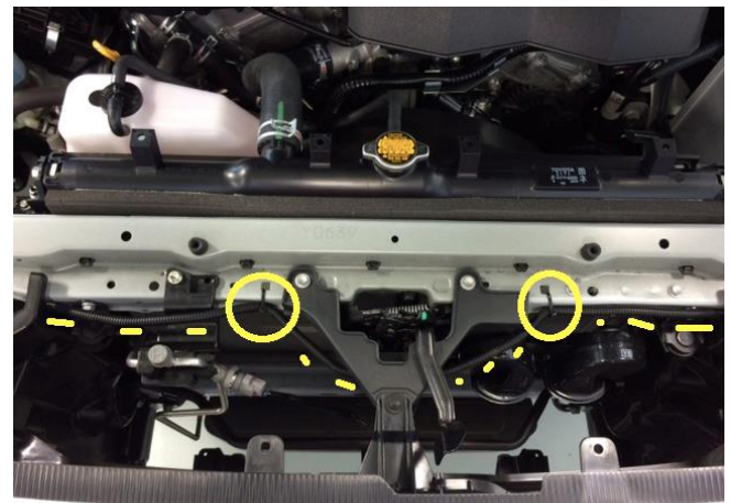
Picture 15B: Securing harness under the hood latch
