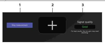
1. **Start/Stop Measurement** – Press this button to start the measurement. An audio test signal will play in your system, after a short warning.
