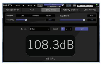
The SPL display allows you to the measure the Sound Pressure Level of your system using a reference microphone. You can investigate the overall SPL in your system, and in different parts of the room for example, alowing you to adjust the system for audience pleasure and audience hearing safety.
