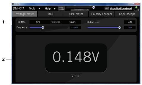
The voltage meter will give an accurate reading of the AC Voltage (rms) of sine wave audio signals entering the DM-RTA.
