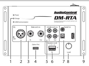
1. **Power LED** – This indicates when the DM-RTA Power switch is turned on. The DM-RTA can be powered by the supplied power adapter, or it can run for up to 4 hours on its internal rechargeable battery.
