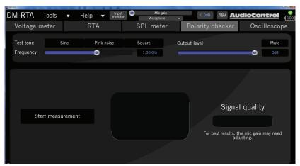
The Polarity Checker display allows you to measure the polarity of the speakers in your system using a microphone. This will allow you to locate any speakers that are wired out of phase. Not that it was you that wired them that way, of course. This is a no-guilt operation designed to help you fix the problem quickly before anyone notices.
