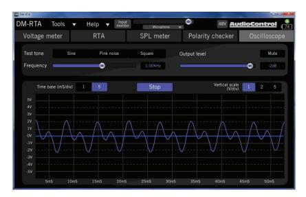
The Oscilloscope display allows you to measure the variation of your incoming audio signal level with time. This will allow you to identify many qualities of your system, for example if the output from your amplifier is distorted in any way (clipping) from the nice signals you are putting in.
