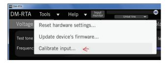
This calibration routine allows you to enter a sine wave of known voltage. The DM-RTA will measure this reference signal and adjust the displayed reading to be exactly the voltage you entered.
