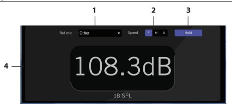
1. Reference Mic – This pull-down menu allows you to select the microphone, so its known properties will be used in the SPL calculations. Select "Other" if your microphone is not listed.
