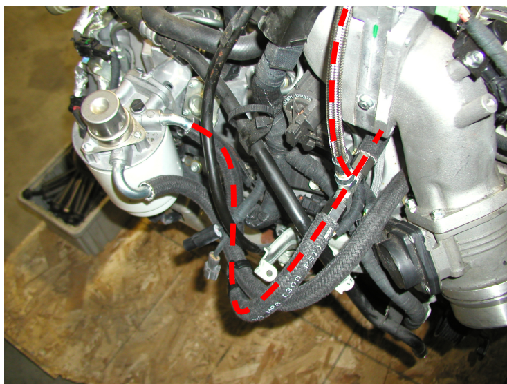
Figure 17: Fuel Supply Tee Installed
