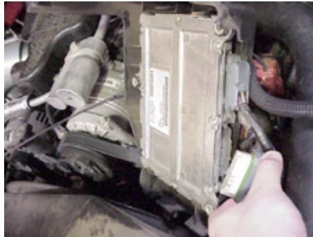
Figure 17: Removing electrical connector
