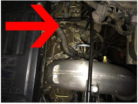
Here you can see the factory wiring harness and connector plugged into the MAP sensor
