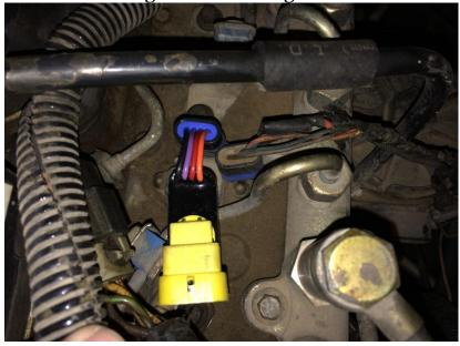
Plug the black connector on the Boost Fooler into the MAP Sensor as shown. (Make sure to tap any wires from a power module or Co-Pilot into the Boost Fooler for best results)
