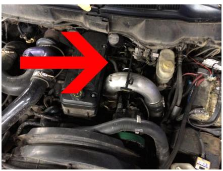
The sensor is located just behind the intake horn to the right of the valve cover.
