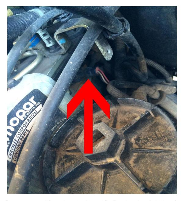
The MAP sensor is located on the driver side of engine, directly behind the factory fuel filter towards the firewall.
