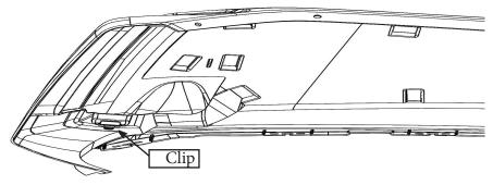
**STEP 6.** Before re-installing the fender onto the jeep, trim off the tabs that once held the fender together. Next either using the clips we removed in step 4 or the optional hardware, re-install the flare. Also trim off the tab on the front of the fender flare that is closest to the body of the jeep.
