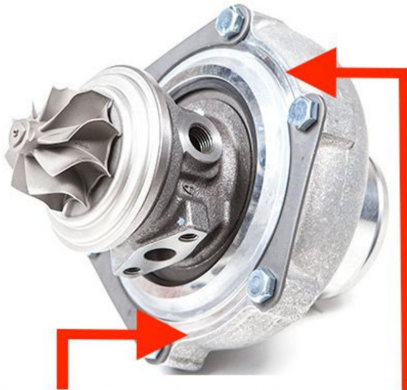
Compressor Hsg. & Backplate Contact Region (Minimal Leakage)
