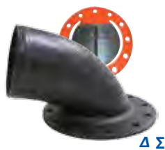
TF689-570 Ultra-Quick Fill Neck w/ "Paddle Valve" TM 4-3/4" B.C., 12 Hole, 3" O.D. Fill, 45°
