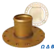
TF222-742 Quick Fill Neck w/ "Paddle Valve" TM 4-3/4" B.C., 12 Hole 2-1/4" O.D. Fill, Straight
