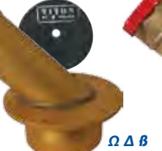
TF184A Quick Fill Neck w/ "Flapper-Valve" 4-3/4" B.C., 12 Hole 2-1/4" O.D. Fill, 45°
