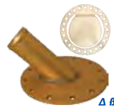
TF669-742 Ultra-Quick Fill Neck w/ "Paddle Valve" TM 4-3/4" B.C., 12 Hole 1-1/2" O.D. Fill, 45°
