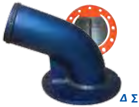
TF523-570 Ultra-Quick Fill Neck w/ "Paddle Valve" TM 4-3/4" B.C., 12 Hole (x2), 2-1/2" O.D. Fill, 22°
