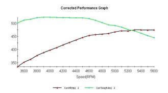
**Cam Specs:** 235/238 @50 .573in/.582ex 112LSA **Cylinder Heads:** Dart Pro 1 62cc/195cc 2.02/1.60 **Rocker Arms:** Aluminum 1.6 Roller Rockers
