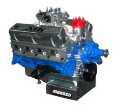
HP: 480 @ 5400RPM TQ: 495 @ 4000RPM Block: OE Ford Roller Block Bore/Stroke: 4.040 x 4.000 Crankshaft: Scat 4340 Forged Rods: Scat 4340 Forged H Beam Pistons: Forged 10.1 Compression
