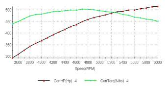
HP: 500+ @ 5800RPM TQ: 515+ @ 4400RPM Block: Seasoned OE Block 4 Bolt Main 1pc Seal Bore/Stroke: 4.040 x 3.750 Crankshaft: Scat 4340 Forged Crankshaft Rods: Scat H Beam Rods W/ ARP Rod Bolts Pistons: Forged 10.1 Compression Rings: Moly Camshaft: Howards Hyd. Roller
