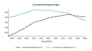
HP: 660+ @ 5300 RPM TQ: 690+ @ 4000 RPM Block: Dart 4 Bolt Main 2pc Seal Bore/Stroke: 4.500 x 4.250 Crankshaft: Manley 4340 Forged Rods: Manley H Beam Rods W/ ARP Rod Bolts Pistons: Forged Flat Top 10.1 Compression Rings: Moly Camshaft: Hyd. Roller
