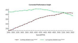
**HP:** 435 @ 5300RPM **TQ:** 475 @ 4200RPM
