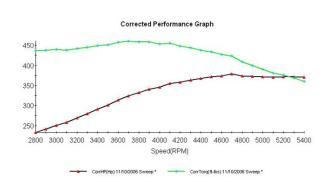
**HP:** 375 @ 4700RPM **TQ:** 460 @ 3800RPM
