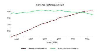
HP: 410 @ 5400RPM TQ: 420 @ 4000RPM Block: OE Ford Roller Block Bore/Stroke: 4.040 x 3.400 Crankshaft: Scat Nodular Steel Rods: Scat 4340 I Beam
