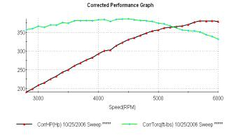
**Cam Specs:** 220/224 @50 .512in/.512ex 112LSA **Cylinder Heads:** Edelbrock Aluminum 60cc 2.02/1.60
