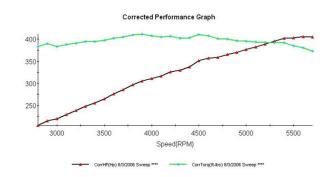
**HP:** 385 @ 5400RPM **TQ:** 390 @ 4000RPM **Block:** OE Ford Roller Block **Bore/Stroke:** 4.040 x 3.500 **Crankshaft:** OE 1pc 28oz Balance
