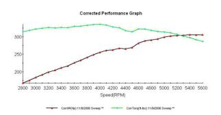
Cam Specs: 219/219 @50 .498in/.498ex 112LSA Cylinder Heads: OE E7TE 62cc 1.77/1.46 Rocker Arms: Stamped Steel 1.6 Rockers
