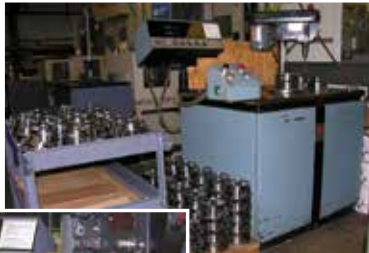
Precision balancing of heavy duty carriers
