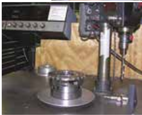
Precision balancing of heavy duty carriers
