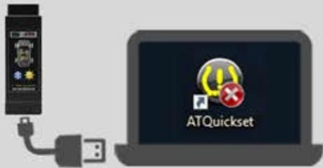
Connect your Quickset tool to your computer via USB cable and open the ATQuickset software.
