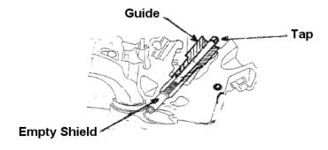
4) Once the ground electrode is tapped, insert the extractor through the guide and thread into the ground electrode shield. Place nylon washer and jam nut onto threaded shaft.
