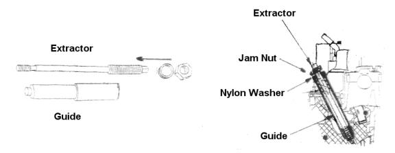
5) While holding hex end of extractor with wrench, turn jam nut with another wrench to remove ground electrode shield.
