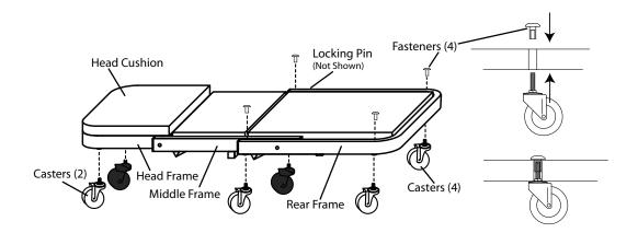
Figure 1 - Model ATD-81045 Components
