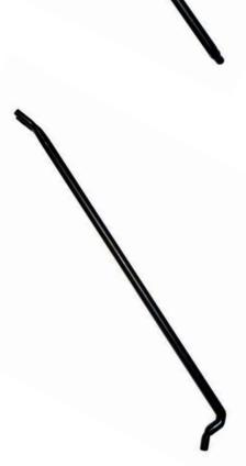
An S-shaped device on the opposite end enables the user to position the brake shoes in a way that allows for leverage for installation of the rollers. The hooked end pulls the brake shoes apart so that the rollers can be installed faster and safely.
