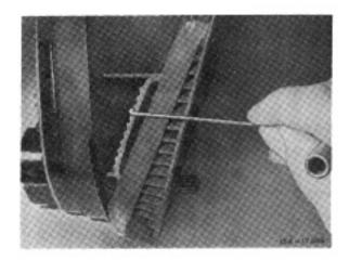
5. Pull instrument cluster out of holder by means of pulling hook. The instrument cluster is held by means of five spring clips located on instrument panel (arrows).
