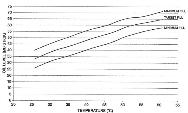
3.0L LE W5A580 Transmission Fluid Fill Curve
