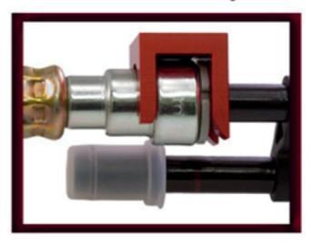
Made of red-anodized aluminum, this power steering & transmission oil cooler line remover is applicable to 1999-2005 BMW 3-Series and X5.
