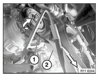
Rotate engine at central bolt in direction of engine rotation.
