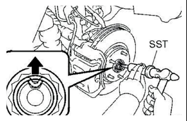
Loosen the staked part of the axle nut completely prior to removing the axle nut
