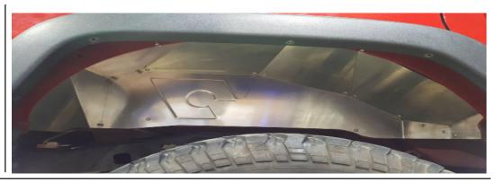
STEP 6. The rear most mounting hole will require drilling to install the hardware. Some choose not use this hole to reduce install time. If you choose not to use this mounting hole the flare will not require removal. We like to use this hole to ensure there is no chance of rattling. Referencing from the back mounting position mark and drill the hole using a 1/4" drill bit. Finish by installing the bolt and nylock locking nut.
