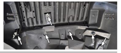
STEP 4. Mark the holes that need to be drilled for rivet nut install. Center punch holes and drill using a 11/32 drill bit. Drilling the hole closest to the firewall can be done from the back side of the flange. (On the passenger side unclip the wiring to provide room for the drill.)
