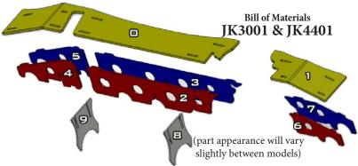
STEP 1. Unpack contents of shipment. Remove axle from vehicle for best results and easiest installation. Prior to mockup make sure axle is clean and uninstall any oem and aftermarket bolt-on accessories that may conflict with truss installation. Remove axle breather hose and uninstall any electric locker wires from casting. This area will be welded so care should be taken to prevent these components for melting.
