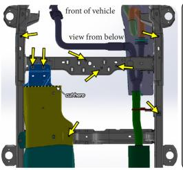
STEP 2A. FOR BEST RESULTS, USE AN ARTEC HD CROSSMEM-BER TO ACHIEVE A TOTALLY FLAT BELLY. If using an Artec HD Crossmember, uninstall the factory crossmember by supporting the transfer case with a jack or straps. Unbolt the internal bolts in the crossmember holding the transfer case. Unbolt the bolts holding the crossmember to the frame and remove the factory crossmember. Install the Artec HD Crossmember using the reverse method.
