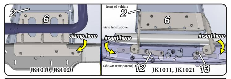
STEP 5. Attaching part 6 is different between the models. See below for model specific instructions.
